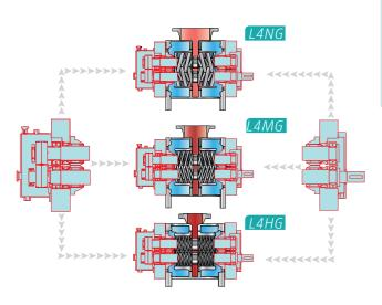
Instead of individual designs, all pumps are designed and manufactured as a modular system. While pump casings, liners and screws are still adapted to the particular operating conditions, bearing covers, bearings, timing gears and the seal components are interchangeable among pumps of different sizes.
