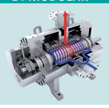
Leistritz screw pumps of series L4 are twin screw double volute, self-priming positive displacement pumps for low, medium and high pressure duty, suitable for transport of abrasive/non abrasive, corrosive/non corrosive, lubricating/non lubricating, high or low viscous fluids.
