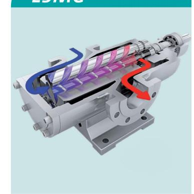
Leistritz screw pumps of the L3MG series are triple screw single volute, self-priming positive displacement pumps for medium pressure duty, suitable for transport of non abrasive, lubricating fluids.
