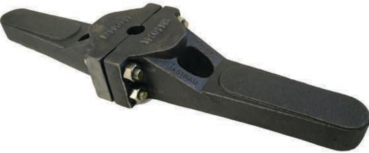
'B' series tillers are supplied ready for final machining to the equipment in your particular vessel – with pilot bore for rudder stock and dimpled for the location of the tiller pin.
